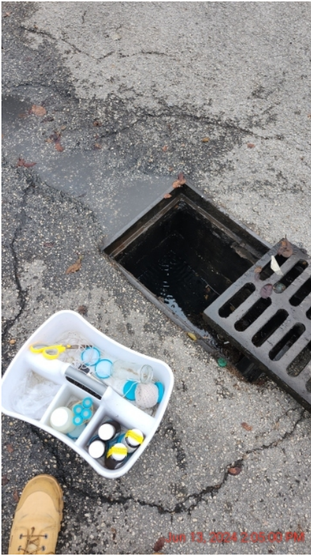
Photo 28: The following samples were collected from the storm drain: VOC (Bluecard #341475), PAH (Bluecard #341476), FL Pro (Bluecard #341477), and Metals (Bluecard #341478).
